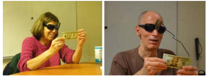
Fig. 8. Evaluation of the proposed system by blind subjects. The bill to be recognized is held by hands and image captured by a camera mounted on a pair of sunglasses.
