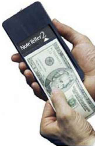
Fig. 2. Portable bill recognition product for blind users in the market “Note Teller 2” [26].
