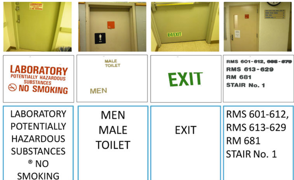
Fig. 12 Top row detected doors and regions containing text information. Middle row extracted and binarized text regions. Bottom row text recognition results of OCR in text regions
