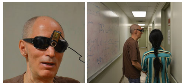
Fig. 15 Example of a prototype system includes a Logitech web camera with auto focus on sunglasses
