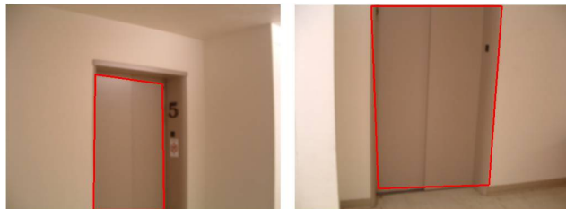
Figure 4. Door detection results under different occlusion conditions. Left: Door detection result with the bottom part occlusion. Right: Door detection result with the top part occlusion.
